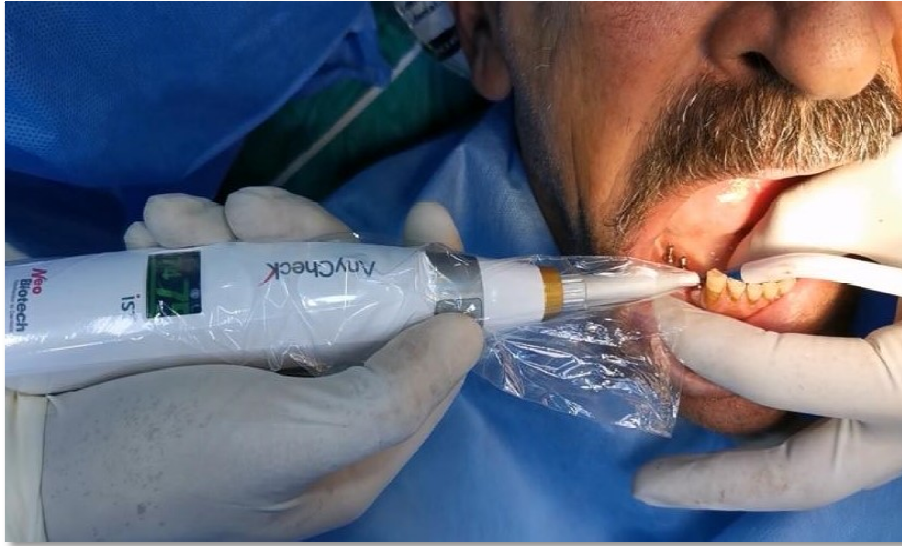
Figure 4. Shows Anycheck device that is used for measuring implant stability.
